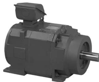
25 HP @ 1150 rpm, L3203 Frame TENV 1000:1 Constant Torque
